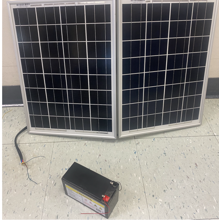
Figure 5.5 Solar Panel and Battery Input Sources
